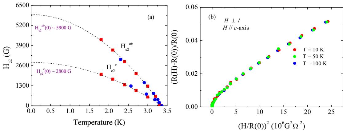
**Fig. 2** (a) Upper critical field  $H_{c2}$  for fields perpendicular and parallel to the  $ab$ -plane as a function of temperature. ( $\blacksquare$ ) and ( $\bullet$ ) were determined by  $R(H)$  at various  $T$  and  $R(T)$  at different  $H$ , respectively. (b) Normal-state transverse magnetoresistance ratio versus  $(H/R(0))^2$  plot at various temperatures. It is interesting to note that all the data collapse onto a universal curve.
