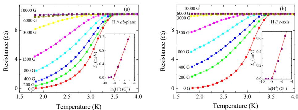
**Fig. 1** Resistance as a function of temperature of InN film deposited on nitridation buffer layer with field in the *ab*-plane (a) and along the *c*-axis (b). The insets display the effective flux pinning energy  $E_a$  versus  $\ln(1/H)$  plots.
