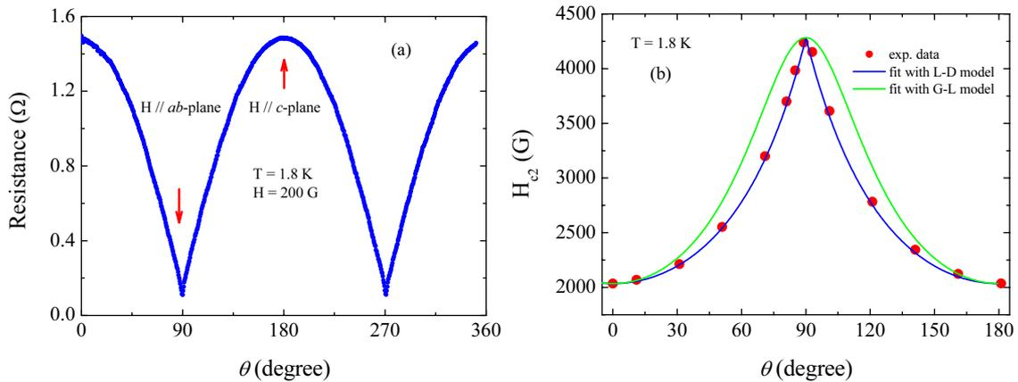
**Fig. 3** (a) Angular dependence of resistance in a field of 200 G measured at 1.8 K. (b) Angular dependence of the upper critical field  $H_{c2}$  at 1.8 K. The solid points are experimental data, whereas the blue and green curves are fitting to L-D and G-L model, respectively.
