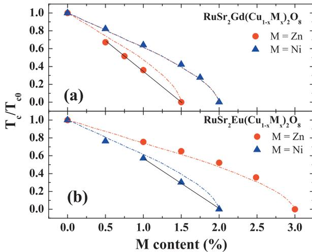
Fig. 2.  $T_c/T_{c0}$  versus impurity content for (a)  $\text{RuSr}_2\text{Gd}(\text{Cu}_{1-x}\text{M}_x)_2\text{O}_8$  and (b)  $\text{RuSr}_2\text{Eu}(\text{Cu}_{1-x}\text{M}_x)_2\text{O}_8$  with  $M = \text{Zn}$  or  $\text{Ni}$ . The dashed curves are obtained by fitting data to A–G formula.
