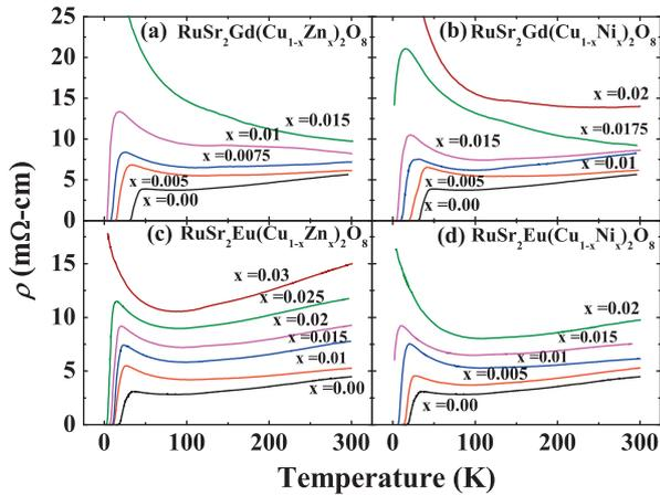
Fig. 1.  $\rho$  versus  $T$  for (a and b)  $\text{RuSr}_2\text{Gd}(\text{Cu}_{1-x}\text{M}_x)_2\text{O}_8$  and (c and d)  $\text{RuSr}_2\text{Eu}(\text{Cu}_{1-x}\text{M}_x)_2\text{O}_8$  with  $M = \text{Zn}$  or  $\text{Ni}$ .
