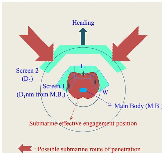
Fig. 3. Basic concept of convoy ASW design. (Source: United States Fleet Anti-Submarine Instructions)
