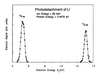
FIG. 1. Spectrum of photoelectrons detached from a fast beam of Li<sup>-</sup> ions by visible radiation from a pulsed laser. The lower-energy and higher-energy peaks are associated with photodetachment via the  ${}^{2}P\epsilon s$  and  ${}^{2}S\epsilon p$  channels, respectively. In the ion frame the  ${}^{2}P\epsilon s$  channel threshold electrons have an energy of 2 meV. This is kinematically "amplified" to about 5 eV in the laboratory frame.
