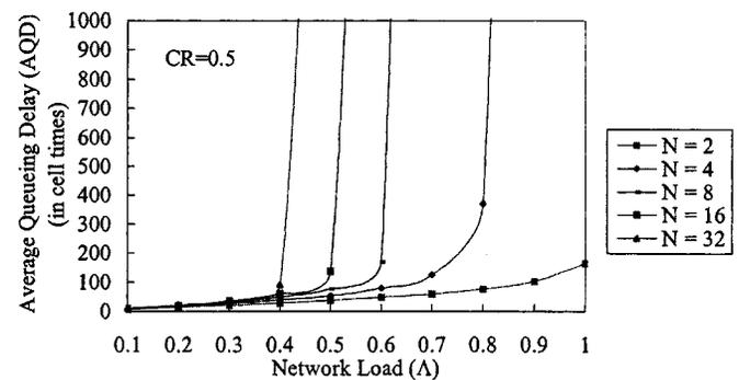
Fig. 10. The AQDs obtained by the CDA under different switch sizes ( $N$ ) and network load ( $\Lambda$ ) when  $CR = 0.5$ .
