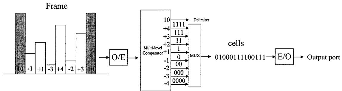
Fig. 5. Structure of Cell Processor (CP).
