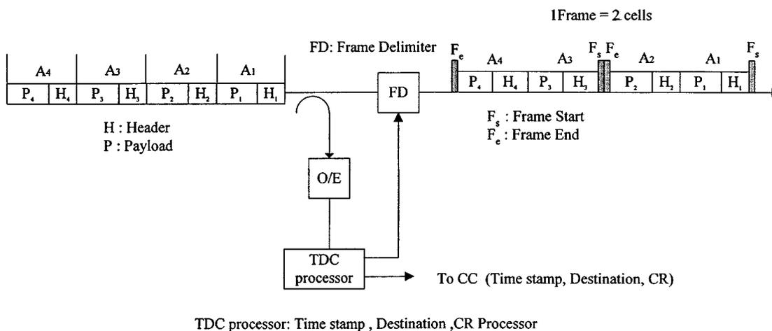
Fig. 2. Structure of Frame Processor (FP).
