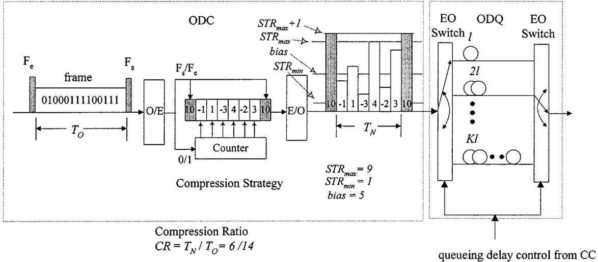
Fig. 3. Structure of ODQ + ODC in smart photonic ATM switch.
