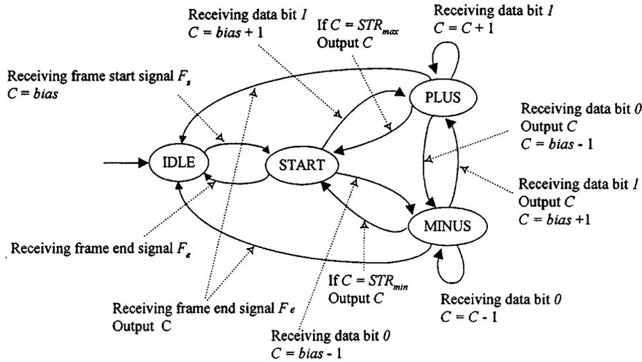
Fig. 4. State transition diagram of compression mechanism.
