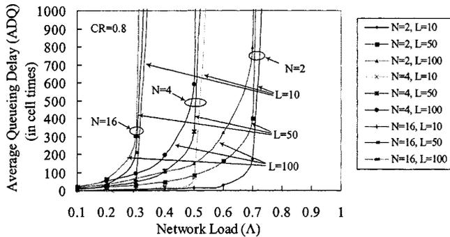
Fig. 11. Comparison of obtained AQQs under different switch sizes ( $N$ ), different frame sizes ( $L$ ) and network load ( $\lambda$ ) when  $CR = 0.8$ .
