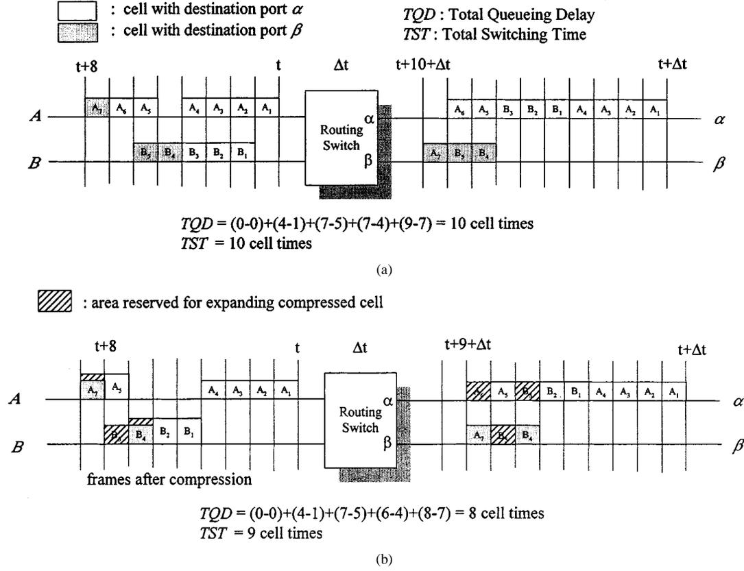
Fig. 6. Example of smart switching method. (a) Traditional switching method. (b) Smart switching method.
