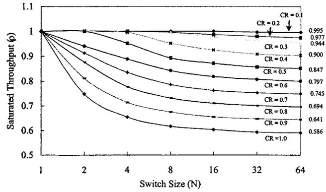
Fig. 8. The obtained throughput of proposed switch architecture strategy under different switch sizes ( $N$ ) and compression ratios (CR) when  $\Lambda = 1.0$ .
