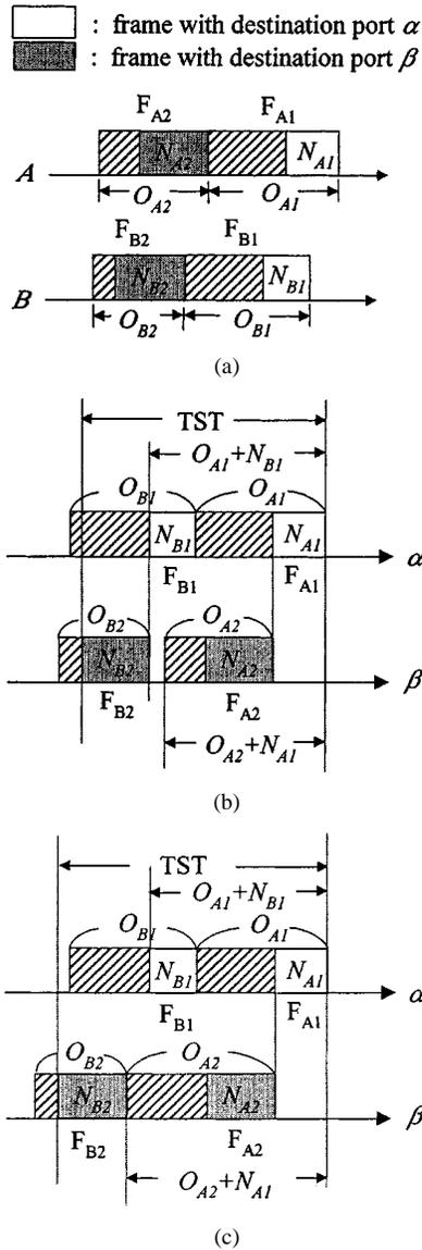
Fig. 7. Performance analysis of proposed CDA. (a) Incoming frames before queuing and compressing. (b)  $TST = O_{A1} + N_{B1} + N_{B2}$  when  $O_{A2} + N_{A1} < O_{A1} + N_{B1}$ . (c)  $TST = O_{A2} + N_{A1} + N_{B2}$  when  $O_{A2} + N_{A1} \geq O_{A1} + N_{B1}$ .
