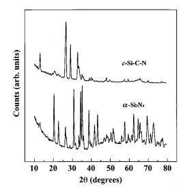
FIG. 1. Representative x-ray-diffraction spectra of polycrystalline *c*-Si-C-N and  $\alpha$ -Si<sub>3</sub>N<sub>4</sub>.
