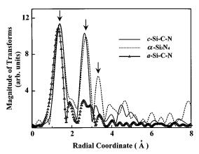
FIG. 6. Magnitude of the Fourier transform of the EXAFS  $k^3\chi$  data of the Si *K* edge of *c*-Si-C-N (solid line),  $\alpha$ -Si<sub>3</sub>N<sub>4</sub> (dashed line), and *a*-Si-C-N (solid line with open triangles) at room temperature.
