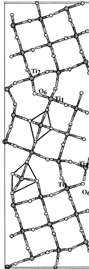
FIG. 4. Atomic structure of the  $\Sigma=15$  tilt boundary in the 60-atom supercell illustrating the Ti-O bonds and the distortion of the oxygen octahedra in the boundary core. The labels  $\text{Ti}^1$ ,  $\text{Ti}^2$ , and  $\text{O}^6$  refer to undercoordinated atoms also shown in Fig. 9.
