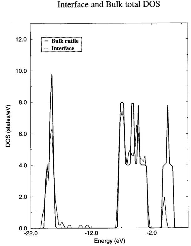
FIG. 7. Total normalized valence band density of states (DOS) at  $(\frac{1}{4}, 0, \frac{1}{4})$  for bulk rutile and the relaxed 60-atom supercell. Note the increased bandwidth in the boundary system. This is consistent with the overall trend towards bond length reduction in the boundary core. A decrease in bond length means that the atoms are pushed closer together, i.e., there is greater orbital overlap than in the bulk, hence a larger bandwidth. The band gap is from  $-2.9$  to  $-0.3$  eV.
