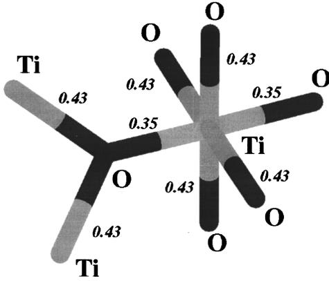
FIG. 8. Bond populations of bulk TiO<sub>2</sub> bonds.
