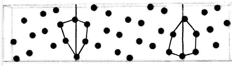
FIG. 3. Relaxed atomic structure of the  $\Sigma=15$  tilt boundary in the 120-atom supercell showing only the oxygen sublattice in the  $z=0$  plane. The 'kite' shaped structural units illustrate the equivalence of the two boundaries in the cell and the mirror symmetry across each boundary plane.
