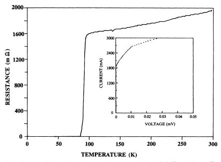
FIG. 1. The electrical resistance of a sample with a nominal composition  $YSrCuO_{4-y}$ . Inset: The *I-V* characteristic at 4.2 K.
