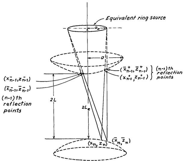
FIG. 8. Equivalent ring source for the  $(n - 1)$ th reflected rays.
