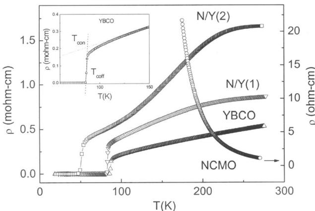
FIG. 2. Resistivity ( $\rho$ ) vs temperature ( $T$ ) for NCMO with the right scale and YBCO, N/Y(1), and N/Y(2) with left scale. The arrows indicate the positions of  $T_{con}$  and  $T_{coff}$  in the inset.
