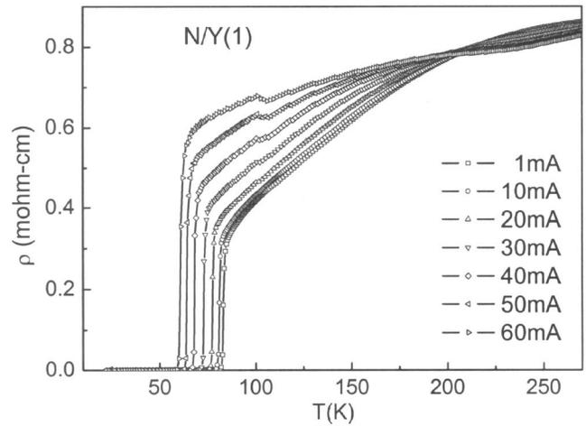
FIG. 3.  $\rho$  vs  $T$  for N/Y(1) with various currents from 1 to 60 mA.
