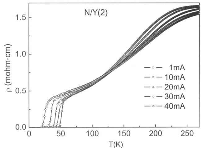
FIG. 4.  $\rho$  vs  $T$  for N/Y(2) with various currents from 1 to 40 mA.
