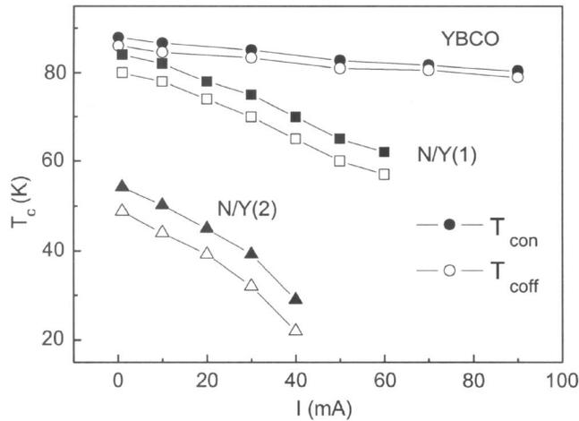
FIG. 5.  $T_{con}$  and  $T_{coff}$  vs current for YBCO, N/Y(1), and N/Y(2).
