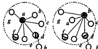
(a) Device *a* plays a master role in the original scatternet. (b) Device *a* executes role switching operation with device *b*.
