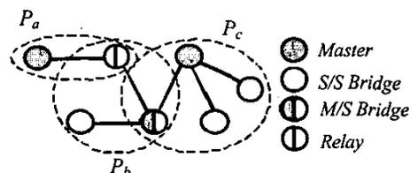
Figure 1: A scatternet consists of three piconets. An S/S bridge connects piconets  $P_a$  and  $P_b$  and an M/S bridge connects piconets  $P_b$  and  $P_c$ .
