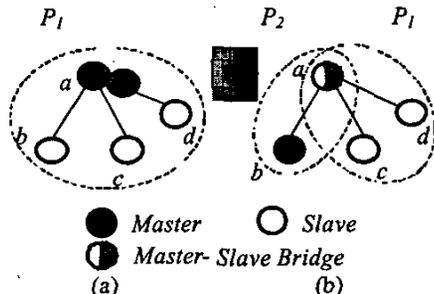
Figure 3: (a) Topology before executing Piconet Splitting operation. (b) Topology after executing Piconet Splitting operation.
