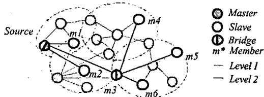
(c) A view of combination of the constructed multicast tree and original scatternet.
