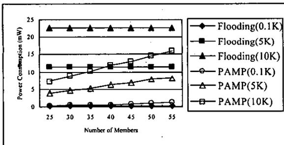
Figure 9: Comparison in power consumptions associated with various data transmission rates.
