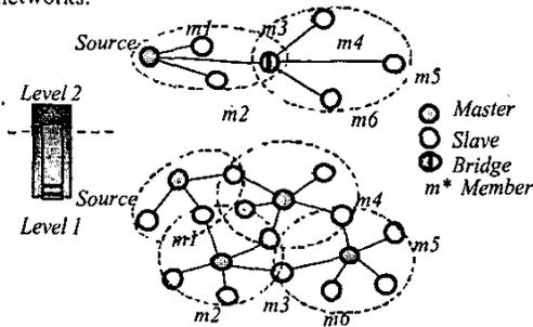
(b) The 2<sup>nd</sup> layer of the Multicast Tree is constructed by the proposed multicast protocol.
