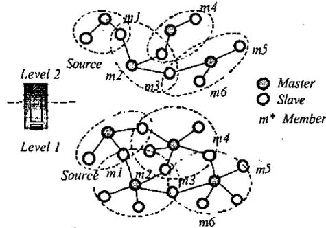
(a) The 2<sup>nd</sup> layer displays the inefficient multicast Tree constructed by flooding based protocol in Ad Hoc networks.
