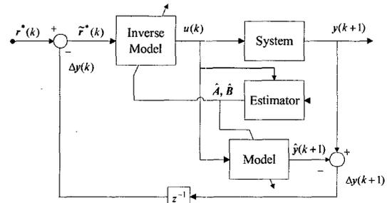
Figure 3 Self-tuning Internal Model Control
