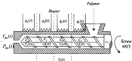
Figure 2 Model configuration of a thermal barrel
