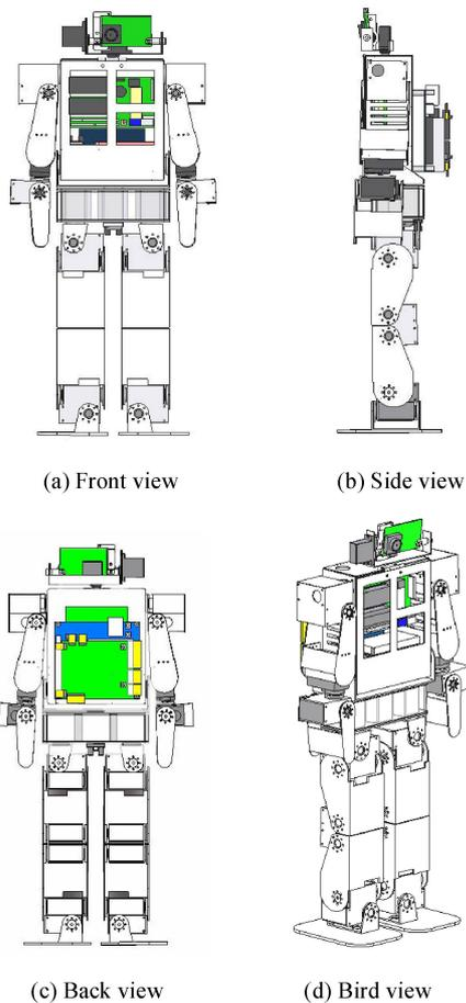
Fig. 3. Solidwork design of TWNHR-3.
