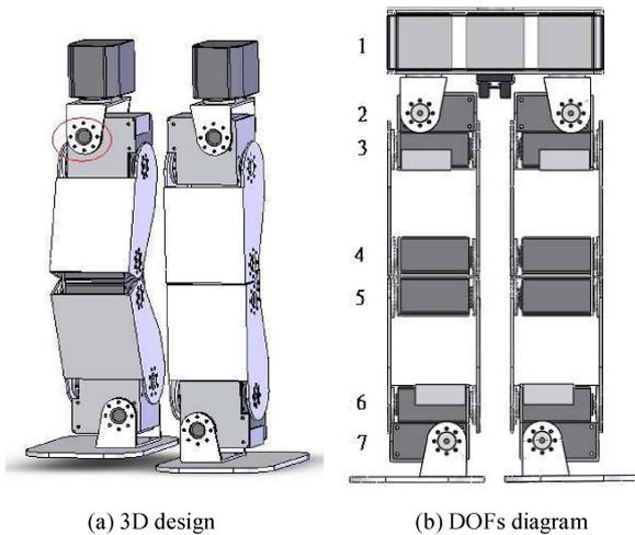
Fig. 7. Legs mechanism.
