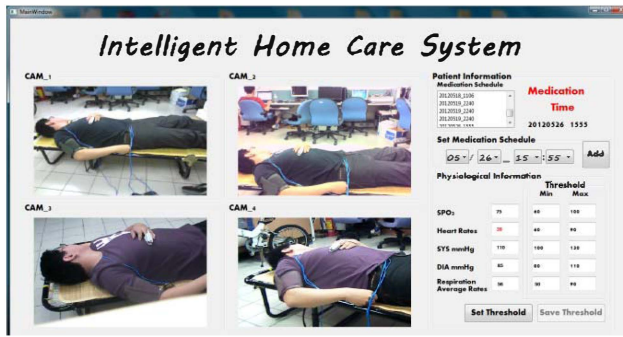
Fig. 3. Web-based interface for the remote monitoring in the proposed system.
