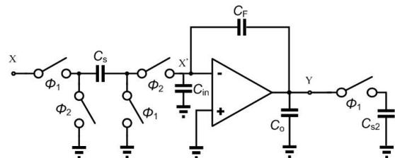
Figure 1. The general SC circuit.
