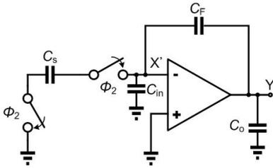
Figure 3. The SC integrator during the slewing and settling phases ( $\phi_2$ ).
