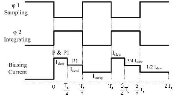
Figure 7. The clock phases of dynamic biasing circuit.
