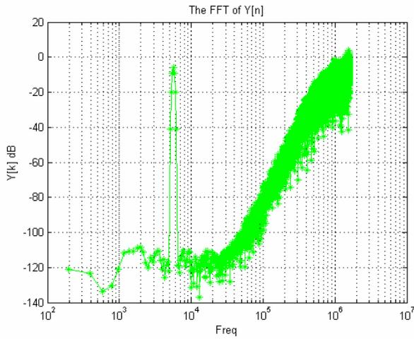
Figure 8. The output spectrum of the modulator
