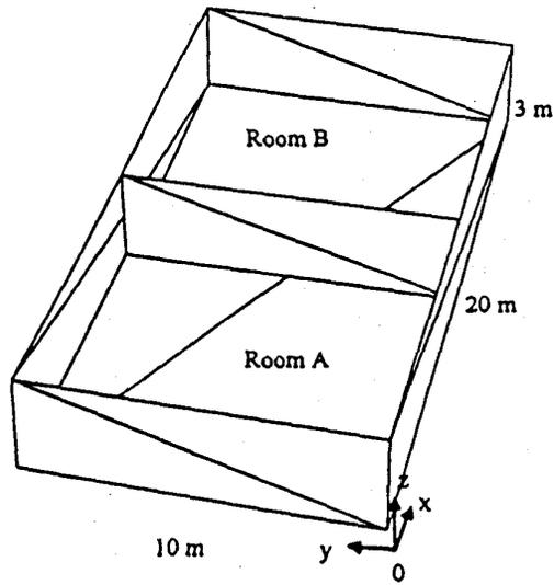
Fig. 1 Two rooms(room A and room B) modeled by triangular facets
