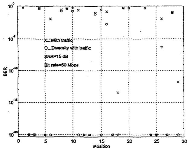
Fig. 9 Dependence of BER on different receiving locations for the case of the tunnel with traffic. SNR is 15 dB and the transmission rate is 50Mbps.
