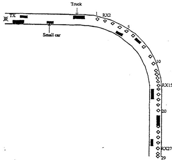
Fig. 4 Top view of the tunnel with traffic. The black rectangles represent the vehicles. TX denotes the transmitter.  $\blacklozenge$  denotes the receiver.
