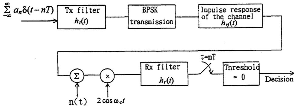
Fig. 2 Block diagram of the simulated communication system.
