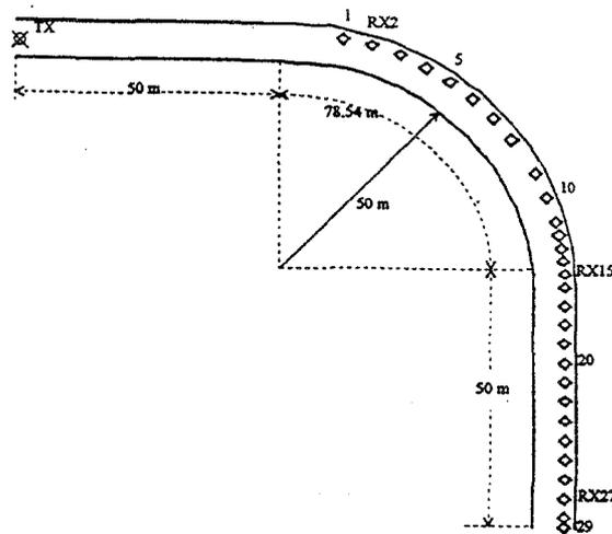
Fig. 3 Top view of the tunnel. TX denotes the transmitter.  $\blacklozenge$  denotes the receiver.
