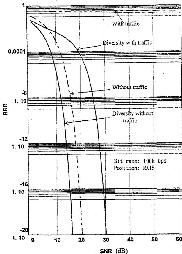
Fig. 7 Dependence of BER on SNR for the cases of tunnels with and without traffic. The transmission rate is 100 Mbps and the receiver is located at RX15.
