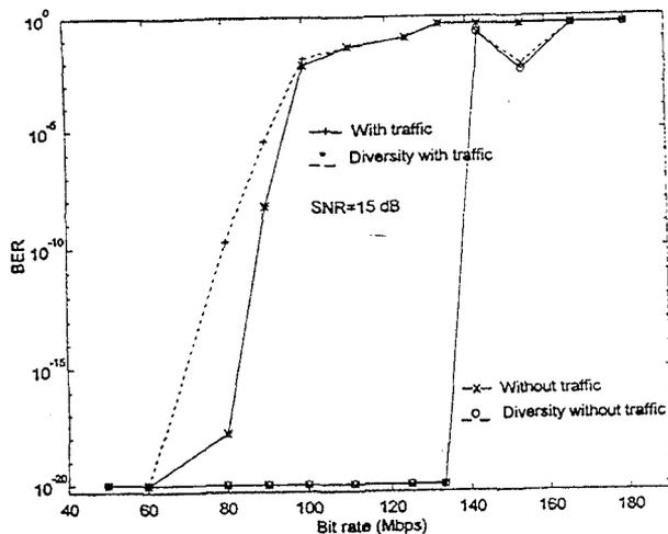
Fig. 8 Dependence of BER on transmission rate for the cases of tunnels with and without traffic. SNR is 15 dB. The receiver is located at RX27.
