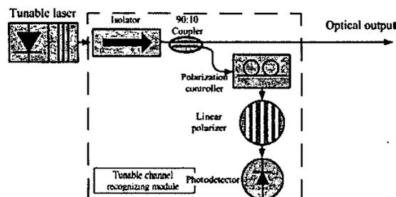
Fig. 1 Schematic of tunable channel recognizing module for a tunable laser
