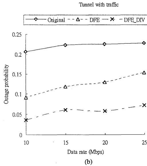
Fig. 6 Outage probabilities versus transmission rate for tunnels with and without traffic and three different receiver structures. (a) for the empty tunnel (b) for tunnel with traffic
