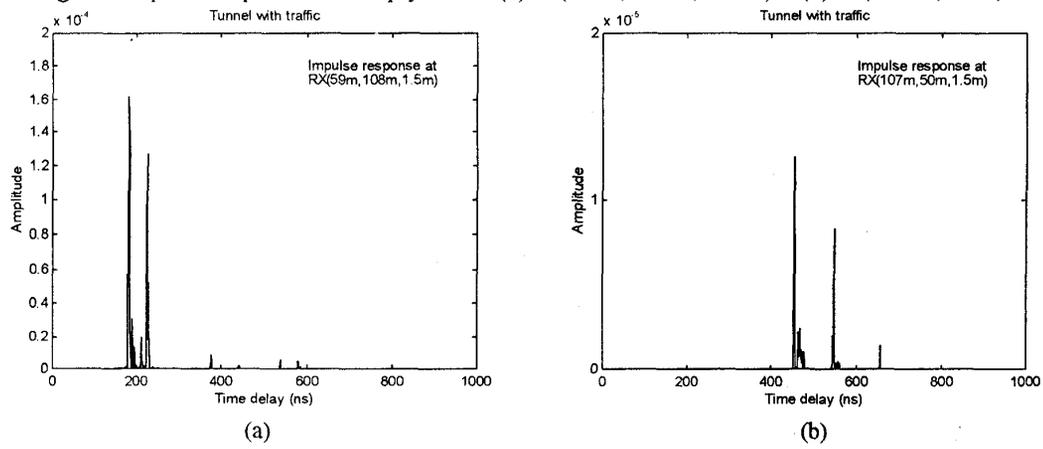
Fig. 4 Impulse responses for tunnel with traffic (a)Rx( 59m, 108m, 1.5m ) (b)Rx( 107m, 50m, 1.5m )
