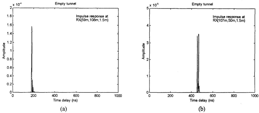
Fig. 3 Impulse responses for empty tunnel (a)Rx( 59m, 108m, 1.5m ) (b)Rx( 107m, 50m, 1.5m )
