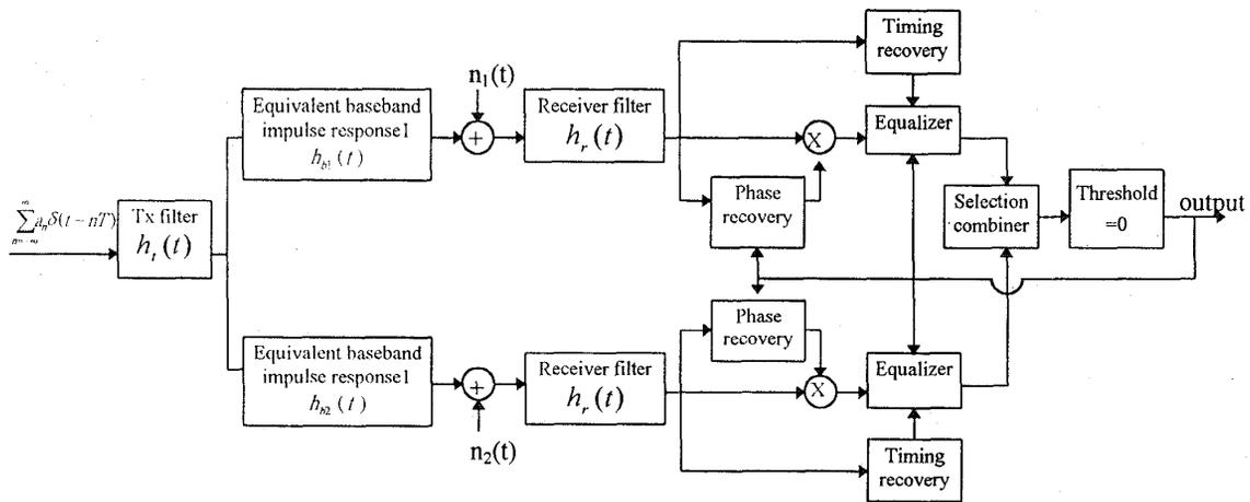
Fig. 2 Block diagram of equivalent baseband communication system with dual space antenna diversity.
