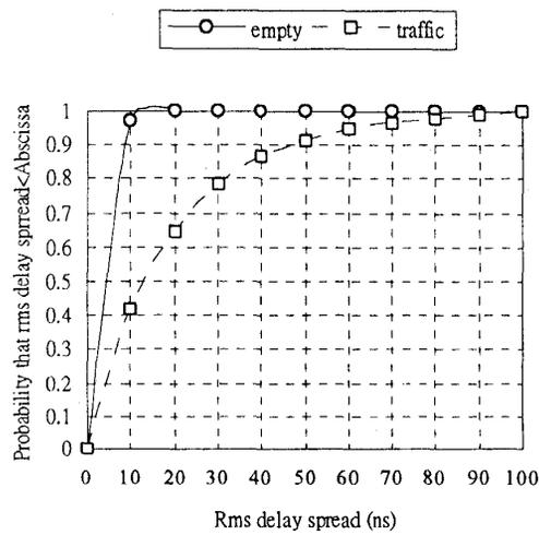
Fig. 5 Cumulative distributions of rms delay spreads for tunnels with and without traffic.
