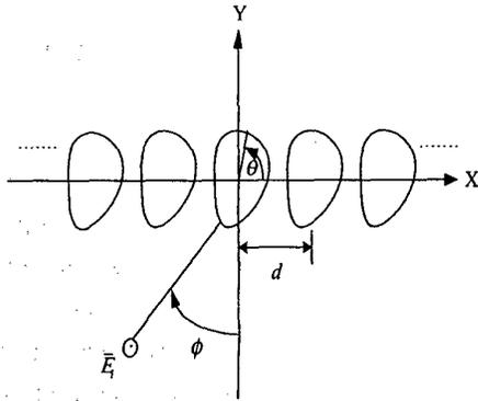
Fig. 1. Geometry of a periodic conducting cylinder with a periodic spacing  $d$  along the  $x$ -direction.
