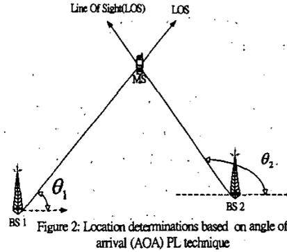
Figure 2: Location determinations based on angle of arrival (AOA) PL technique
