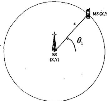
Figure 3 : Location determinations based on Hybrid of TOA/AOA PL techniques
