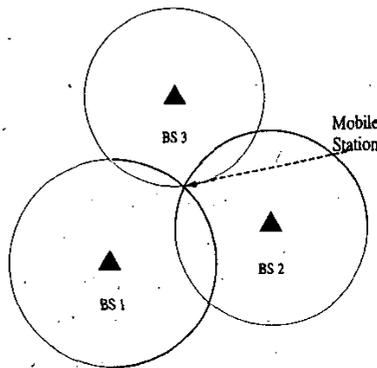
Figure 1 :Location determinations based on time of arrival (TOA) PL technique
