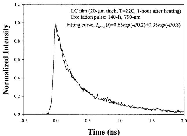
FIG. 3. Measured two-photon-induced fluorescence decay curve (solid line) excited by  $\sim 790\text{-nm}$  and  $\sim 140\text{-fs}$  laser pulses. The dashed line is a double exponential decay curve with two decay constants of  $0.2$  and  $0.8\text{ ns}$  respectively.
