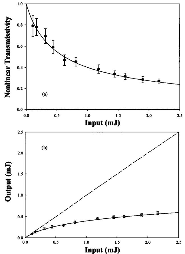
FIG. 4. (a) Measured nonlinear transmissivity data as a function of the input energy; the thick solid line is the best fitting curve with  $\beta=6.25\text{ cm/GW}$ . (b) Measured output energy versus input; the thin solid line is the best fitting curve with the same  $\beta$  value.
