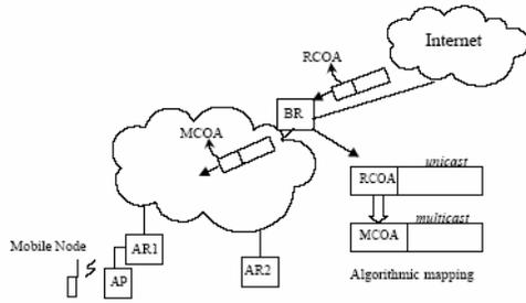
Fig.2: M&M Algorithm Mapping architecture
