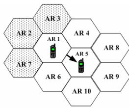
group by MCoA to receive the packets destined to the MN. Hence, the mobile can move to any router in the CAR-set without interrupt\_
