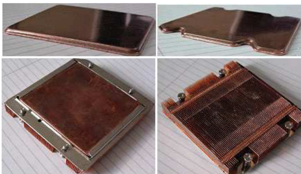
FIGURE 18. Tail-free vapor chamber (Acmeools Electronic Technology Inc.) ( http://www.acmeools.com/ )
