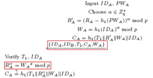
Fig. 10. The original Smart Card authentication packet.
