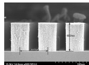
Fig.1. Pattern-less CNT with Grown Height 85  $\mu\text{m}$
