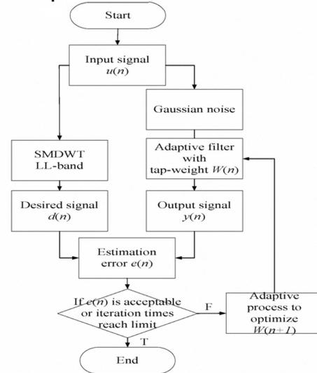
Fig. 3. The training flow by using LMS with DWT operation.
