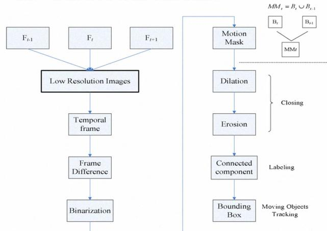
Fig. 1. Flow chart of the moving object detection and tracking by using the low resolution image.
