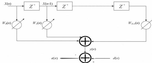
Fig. 2. N-tap transversal adaptive filter.
