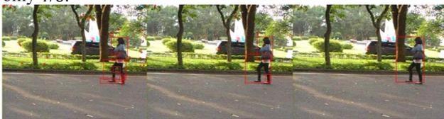
Fig. 4. Results of tracking moving objects in various time with static background: (a) original frames without LMS-based moving objects tracking method, (b) LL<sub>1</sub>-band frames with LMS-based moving objects tracking method, (c) LL<sub>2</sub>-band frames with LMS-based moving objects tracking method.
