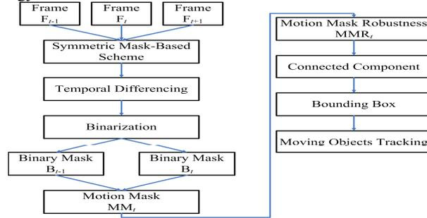
Figure 3. Flow chart of the moving object detection and tracking based on SMBS.
