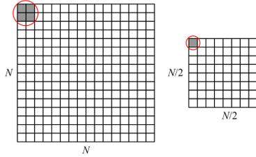
Figure 1. Diagram of the  $2 \times 2$  average filter method.
