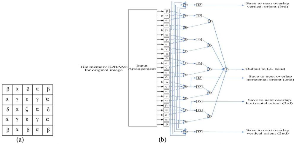
Fig. 2. LL band mask coefficients and the corresponding DSP architecture. (a) Coefficients. (b) Hardware architecture design.
