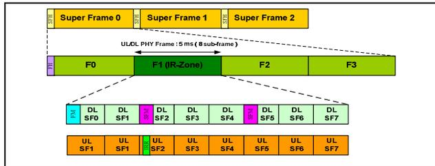
Figure 1 (b) Control channel structure for FDD
