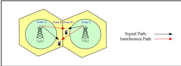
Figure 14 Cell-edge interference
