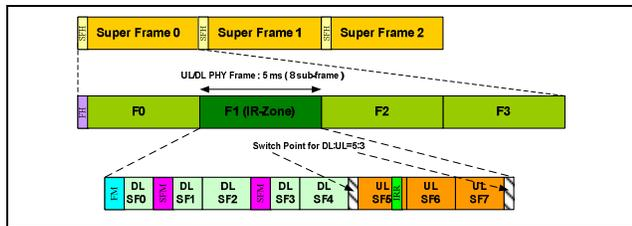
Figure 1 (a) Control channel structure for TDD
