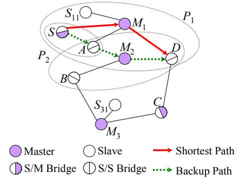
Figure 5: Final route construction phase in LAMP.
