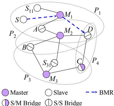
Figure 2: An example of the routing path constructed by BMR between the source  $S$  to the destination  $D$ .
