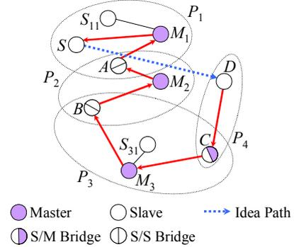
Figure 3: RSP is forwarded along the path from the destination  $D$  to the source  $S$ .
