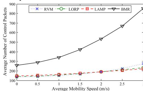
Figure 8: The average number of control packets in different protocols for the different average mobility speed.
