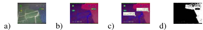
Fig. 3. a) The original figure; b) Transformed to the HSI color space; c) Determine the threshold value; d) Binarization
