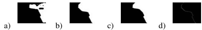
Fig. 4. a) Filtering is applied; b) Dilation is applied; c) Erosion is applied; d) Edge detection to obtain the sea shore.
