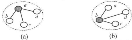
Figure 1: (a) Topology before executing Piconet\_TakeOver(b, a) . (b) Topology after executing Piconet\_TakeOver(b, a) .
