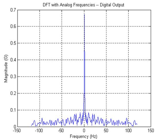
Figure 12. Spectrum distribution of the acceleration signal from digital output.
