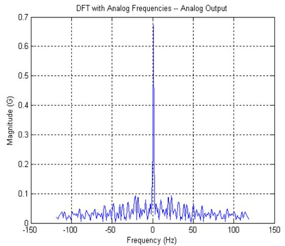
Figure 11. Spectrum distribution of the acceleration signal from analog output.
