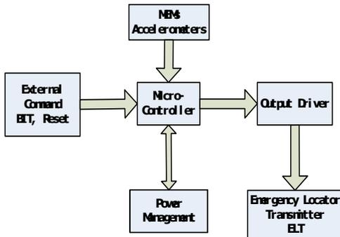
Figure 3. Collision sensor system block diagram
