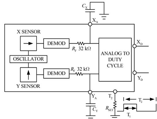
Figure 5. ADXL210E MEMS accelerometer [5]
