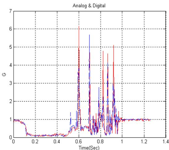
Figure 10. Comparison of the acceleration signals between analog and digital outputs.
