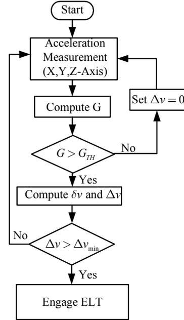
Figure 4. Crash condition determination flow chart
