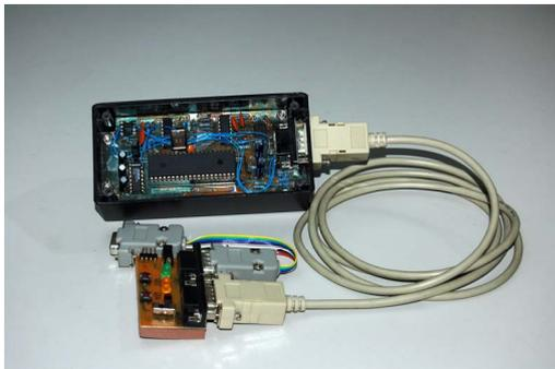
Figure 6. Prototype of the collision sensor
