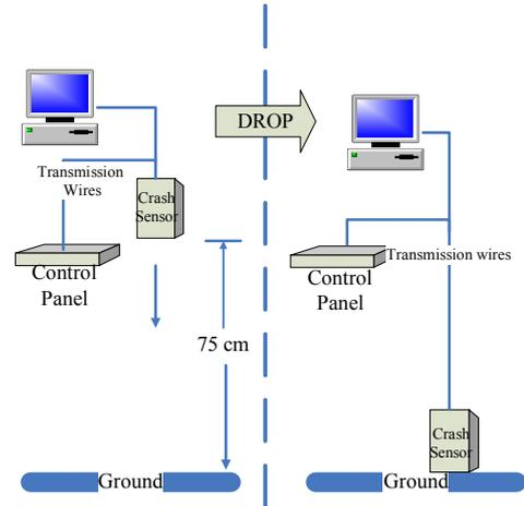
Figure 7. Construction of the drop test
