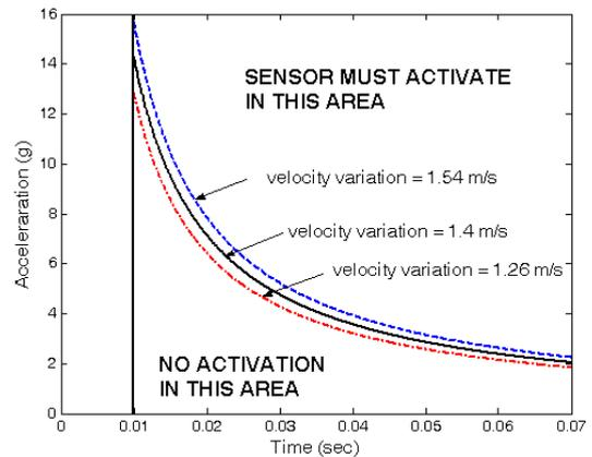
Figure 2. Collision sensor response curve
