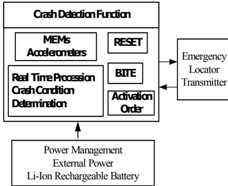
Figure 1. Basic functions of a collision sensor
