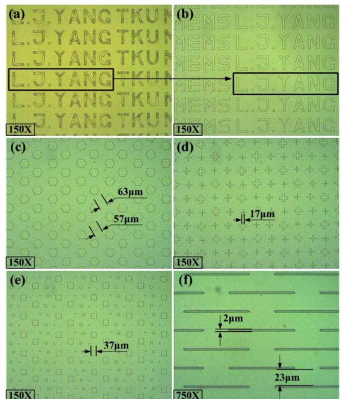
Figure 2. The fabricated gelatin micropatterns: (a) before stripping the photoresist mask; (b) stripping the photoresist, micro letter pattern of 17  $\mu\text{m}$  width; (c) micro honeycomb patterns; (d) micro "cross" patterns, the largest width is 17  $\mu\text{m}$ ; (e) micro square patterns, the largest width is 37  $\mu\text{m}$ ; (f) microstrips lines with 2  $\mu\text{m}$  width, 90  $\mu\text{m}$  length and the gap between two lines is 23  $\mu\text{m}$ .
