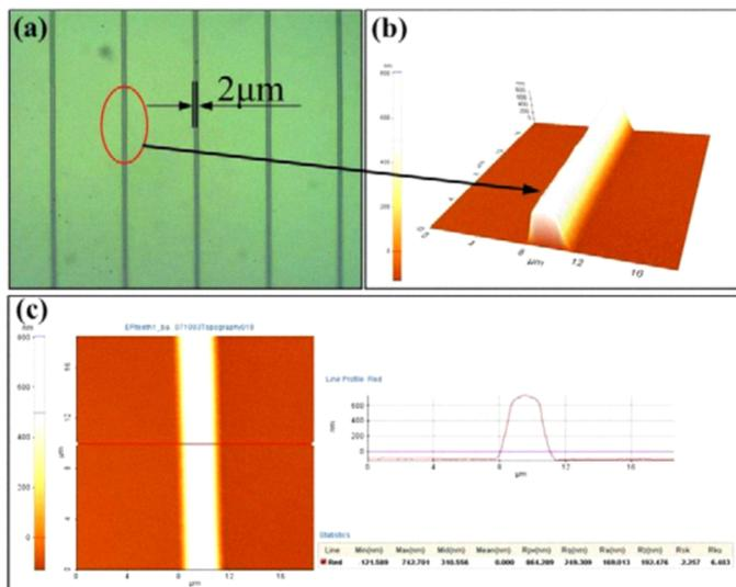
Figure 3. Thickness measurement of gelatin micropattern scanned by AFM: (a) the scanned sample of microstrips lines with 2  $\mu\text{m}$  width; (b) AFM scanning picture of microstrip gelatin; (c) the cross-section line profile of microstrips lines with 0.8  $\mu\text{m}$  thickness.
