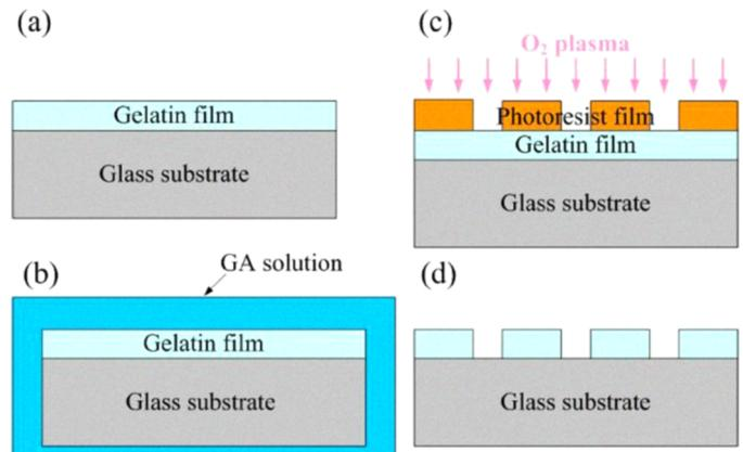
Figure 1. The patterning process of GA-crosslinked gelatin: (a) Spin-coating pure gelatin film at 50 °C, drying for 1 day; (b) Crosslinking gelatin film in 50% GA solution; (c) Patterning a positive-toned photoresist mask on the gelatin film and etching by O<sub>2</sub> plasma; (d) Stripping photoresist by acetone.
