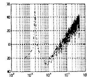
Fig 9. FFT Plot of the Output of the With-Noise  $\Delta\Sigma$ M in Fig. 8
