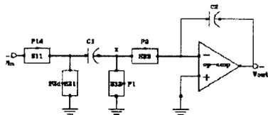
Fig. 6a. The SC Integrator with Phase-Delay Design
