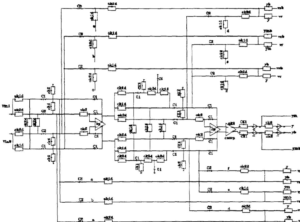
Fig. 7. A Second Order  $\Delta\Sigma$ M with Gain-Compensation, Fully Differential and Phase Delay Design
