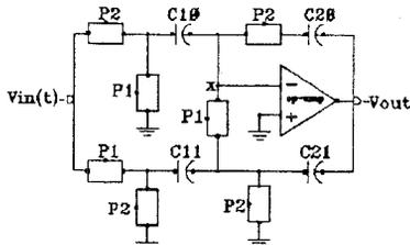
Fig. 3. A Gain-Compensated SC Integrator (GC11) ( $C11=2C10$  and  $C21=C20$ ).
