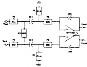
Fig. 5. A Fully Differential SC Integrator
