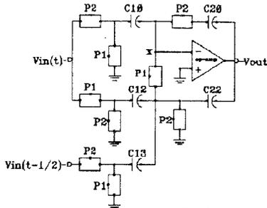
Fig. 4. A Gain-Compensated SC Integrator (GC12) ( $C10=C10=C13$  and  $C20=C22$ ).
