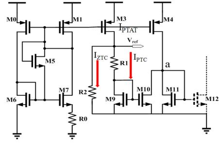
Fig. 1 Temperature compensation current reference
