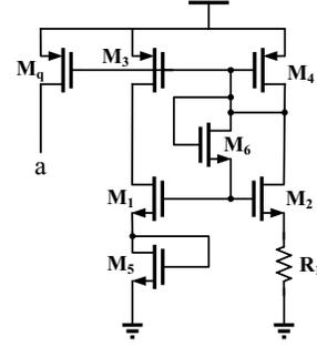
Fig. 2 The opposite characteristic curve temperature independent current reference
