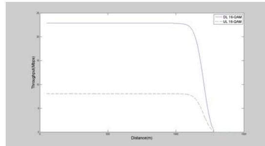
Figure 3 Transmission Efficiency Before Calibration (16 QAM)
