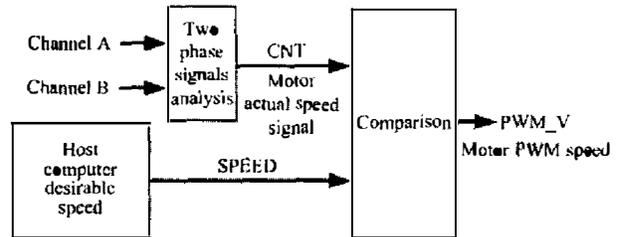
Fig. 8. Design flow diagram of motor feedback controller
