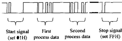
Fig. 4. Serial signals of the multi-control command
