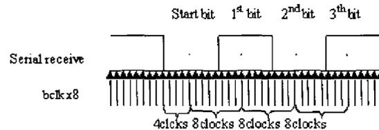
Fig. 3. Asynchronous serial data receiving method.
