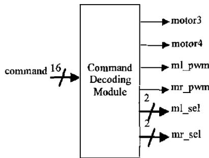
Fig. 6. Block diagram of the command decoding module.
