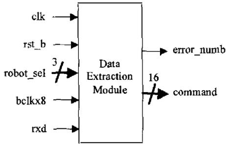
Fig. 5. Block diagram of the data extraction module.
