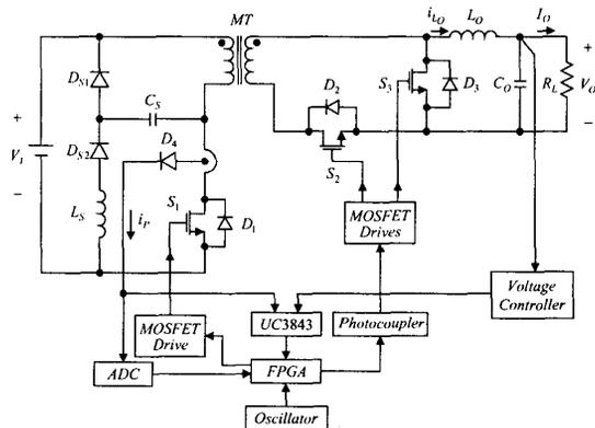
Fig. 1. System configuration of the experimental forward converter.
