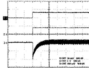
Fig. 12. Transient load response from no to full load with a time scale of 500us/div: (i)  $I_O$  with 15A/div for channel 1; (ii) SRCON with 5V/div for channel 2; (iii) output voltage variation with 100mV/div for channel 3.
