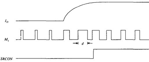
Fig. 4. How to determine states exchange from no to full load.
