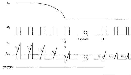
Fig. 5. How to determine states exchange from full to no load.
