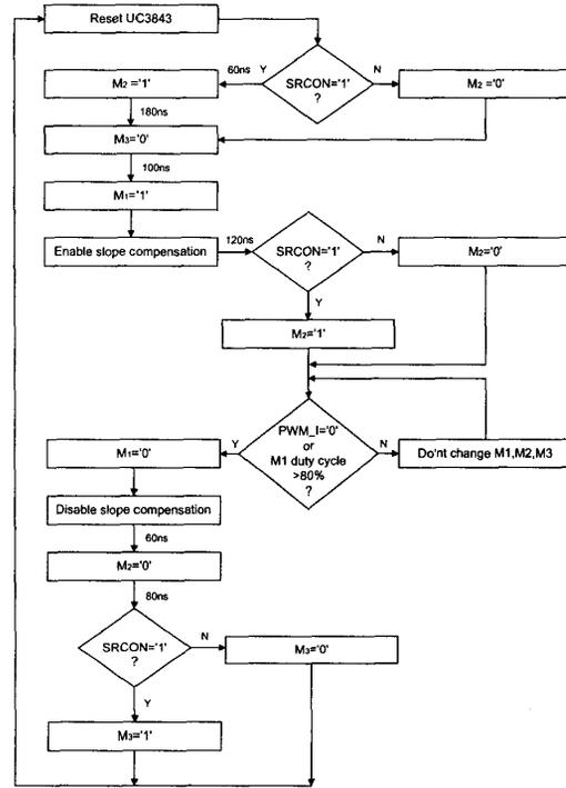
Fig. 7. How to generate the timing sequence for  $M_1$ ,  $M_2$  and  $M_3$  based on SRCON.
