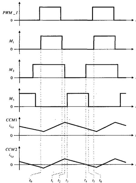
Fig.3. Timing sequences for CCM1 and CCM2 under SR.
