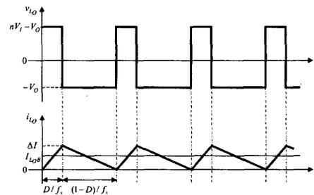
Fig. 2. Current flowing through  $L_O$  on the boundary between CCM and DCM under no SR, along with the voltage across  $L_O$ .
