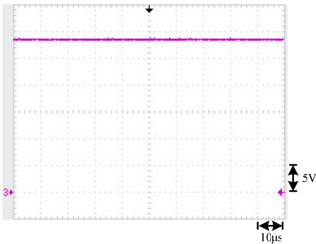
Figure 12. The steady-state output voltage 28V.
