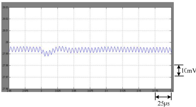
Figure 9. Simulated transient load response due to load change from 0% to 100%.
