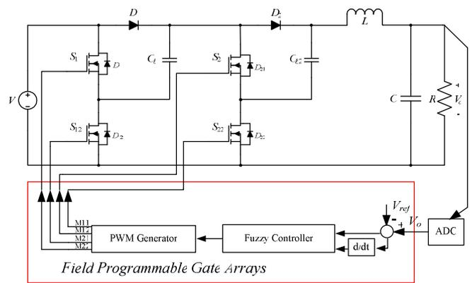
Figure 10. Block diagram of the overall system.
