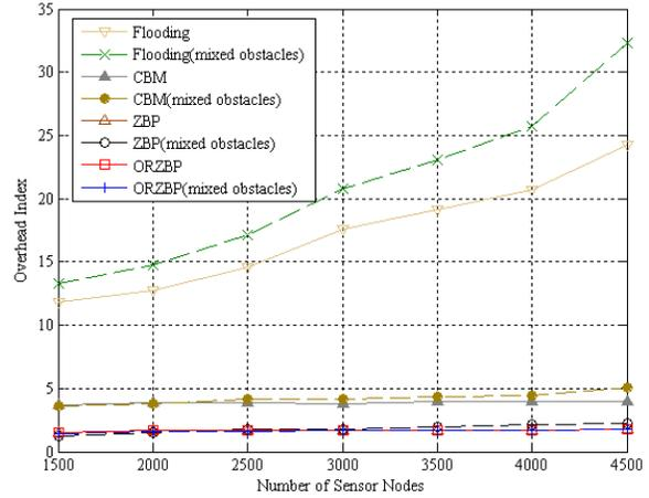
Figure 14: *Overhead Index* with multiple middle-sized obstacles.
