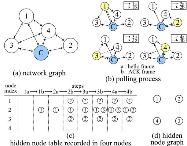
Figure 2. An example illustrates how the coordinator builds the hidden node graph.
