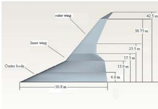
Figure 2. Blended Wing Body geometry model.<sup>12</sup>
