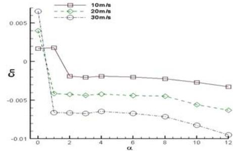
Figure 15. The yawing moment coefficient  $C_n$  vs. AOA at three different crosswinds.
