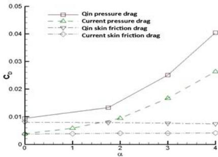
Figure 9. Pressure drag and skin friction drag comparison.
