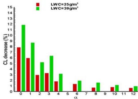
Figure 17. The lift coefficient decrease ratio at two different rain rates.
