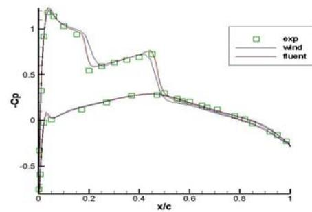
Figure 7. M6  $C_p$  distribution at section  $y/b=0.65$ .
