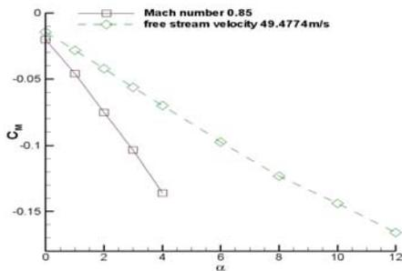
Figure 10. The pitching moment coefficient  $C_M$  vs. AOA at two different velocities.
