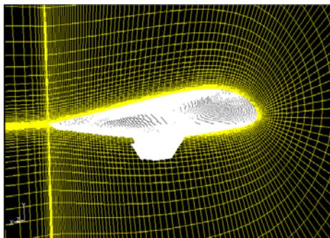
Figure 4. Near mesh of the Blended Wing Body.
