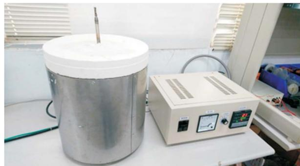
Figure 3. Heat pipe in furnace and power supply.
