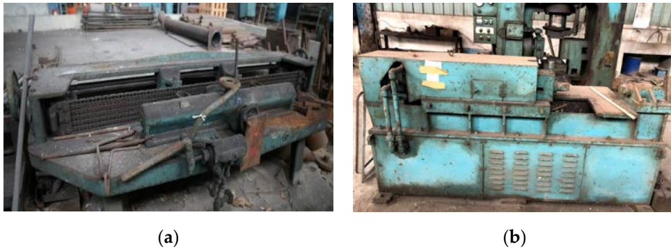
Figure 17. Bending, shaping, and assembling. (a) Spring forming machine (A12), (b) strapping machine (A05-2).
