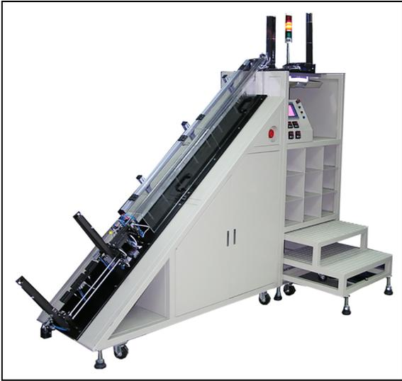
**Figure 1.** Piranha LED automatic thermal test sorting machine.
