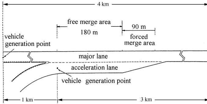
Fig. 2. The layout of a mimicked junction section.
