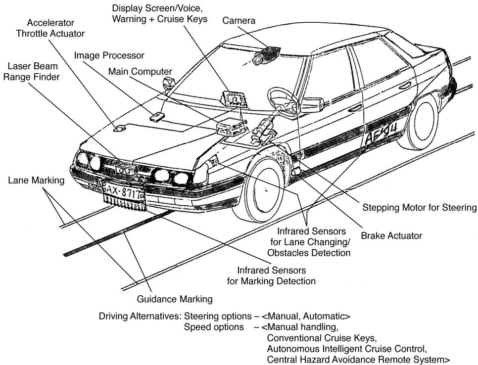
Fig. 1. Scheme of an ADVANCE-F vehicle.
