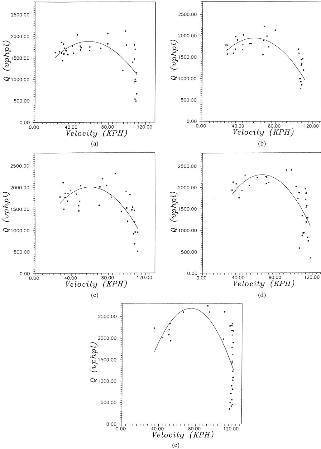
Fig. 5. V-Q diagram (a) mixed ratio 0.0; (b) mixed ratio 0.3; (c) mixed ratio 0.5; (d) mixed ratio 0.8; (e) mixed ratio 1.0.
