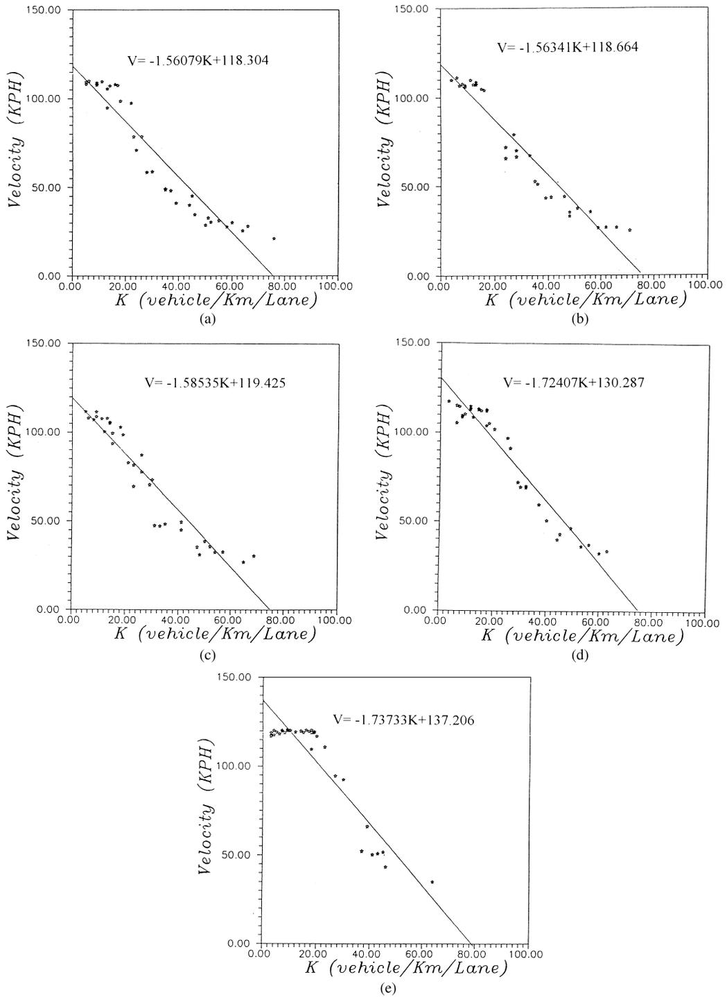
Fig. 6. K–V diagram (a) mixed ratio 0.0; (b) mixed ratio 0.3; (c) mixed ratio 0.5; (d) mixed ratio 0.8; (e) mixed ratio 1.0.
