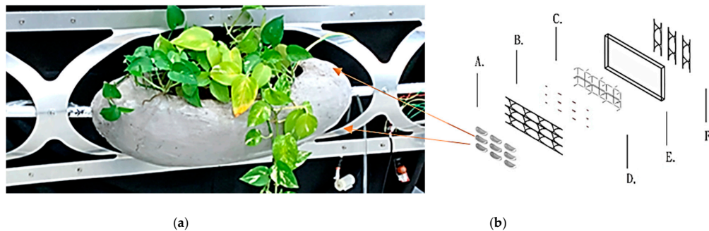
Figure 12. Conceptual development of adding the vertical green system to existing building envelope. (a) full-scale planting cell prototype; (b) is the assembly diagram: A is the plating cell; B is the sub-framing grid; C is the attachment structure; D is the support subsystem; E is the unit frame, and F is the irrigation support. Source: AJL CReS lab Research Studio [106,107].
