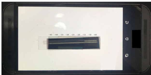
Fig. 7. The image of LC-based immunoassay captured by a smartphone. It shows that the LC image was clear, and the length of the bright LC image can be easily differentiated with an integrated scale bar.
