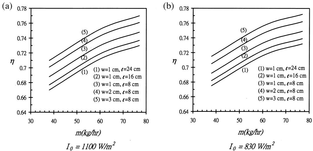
Fig. 7. Effect of baffle density on collector efficiency in baffled solar air heaters of collector aspect ratio 3/2.
