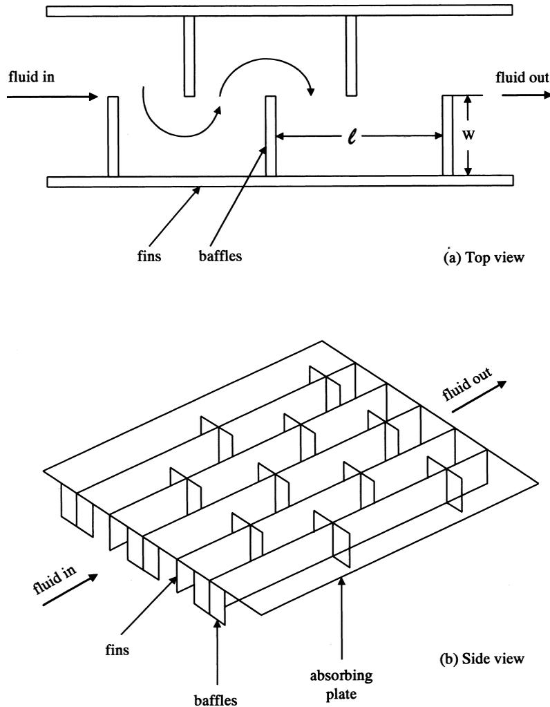
Fig. 2. Fins with attached baffles.
