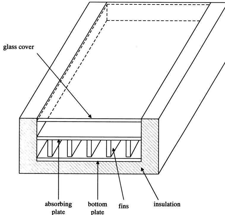
Fig. 1. Solar air heater with fins.
