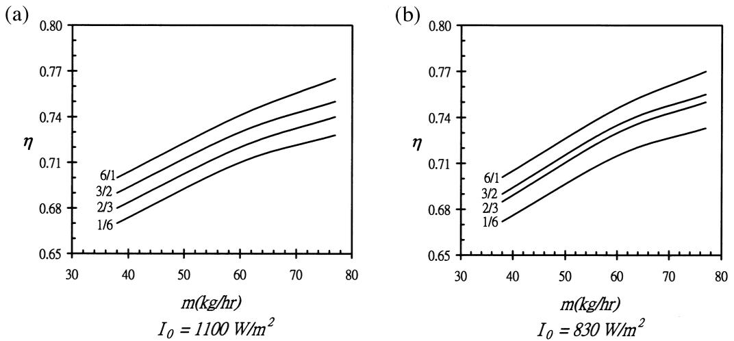
Fig. 5. Effect of collector aspect ratio on collector efficiency in flat-plate solar air heaters with fins attached by baffles.
