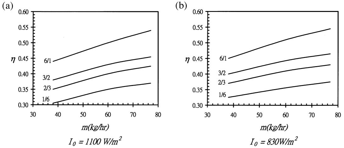
Fig. 3. Effect of collector aspect ratio on collector efficiency in flat-plate solar air heaters.
