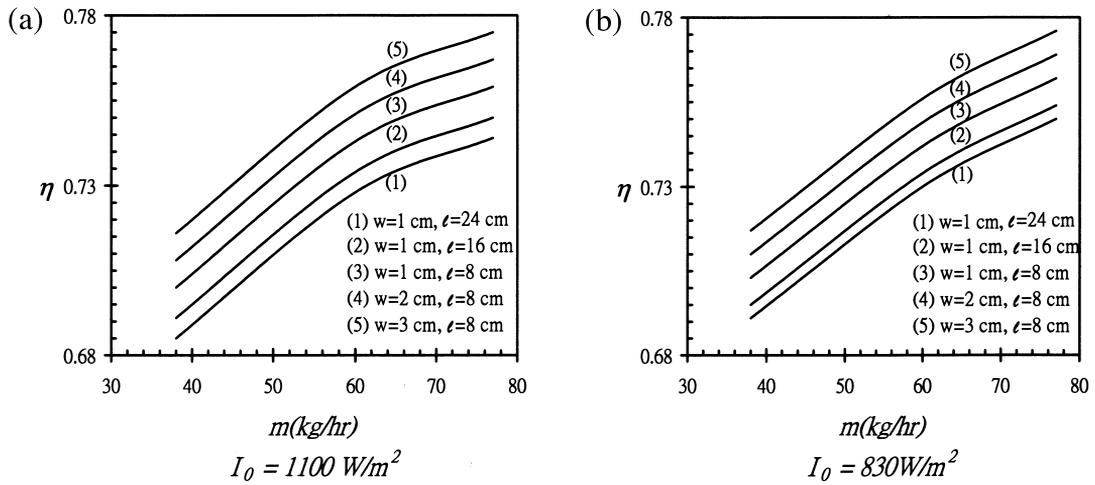
Fig. 6. Effect of baffle density on collector efficiency in baffled solar air heaters of collector aspect ratio 6/1.
