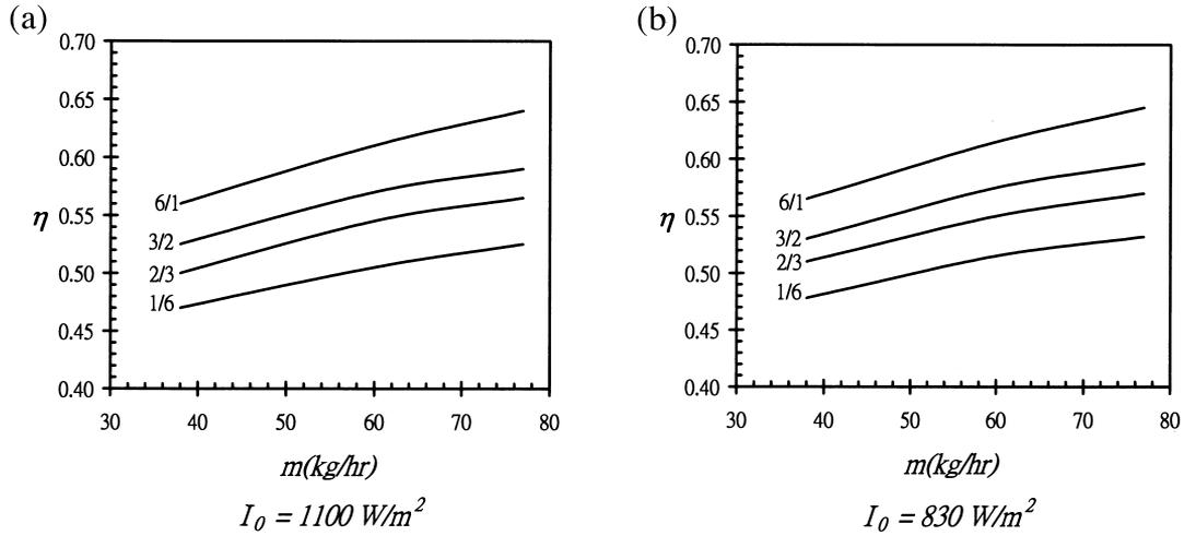
Fig. 4. Effect of collector aspect ratio on collector efficiency in flat-plate solar air heaters with fins.
